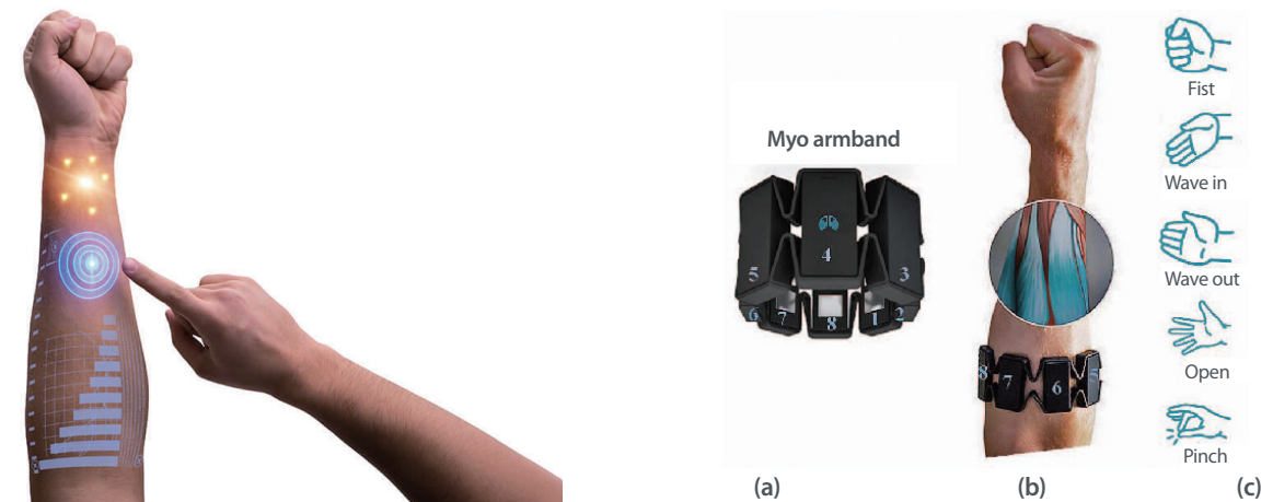
Fig. 1. Myo armband: (a) number of the EMG pods, (b) location on the forearm and (c) gestures to recognize.
